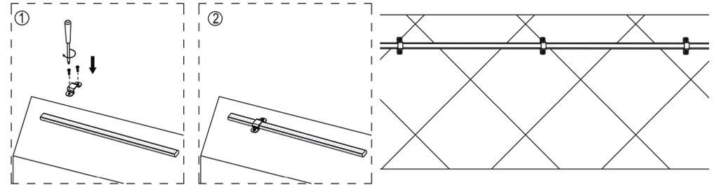
Use suitable clamps or holders for permanent attachment. Do not use thin wire or similar to attach it, as this could damage the plastic coating. In the case of longer or permanent installation, the LED Strip must be fixed vibration-free in order to prevent line breaks.
