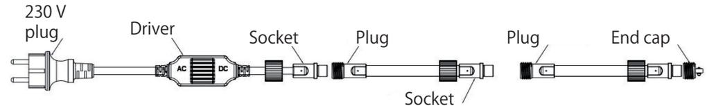
To expand the LED strip, connect the plug and socket together. Please make sure that the union nut and the end cap are screwed correctly and tightly!
